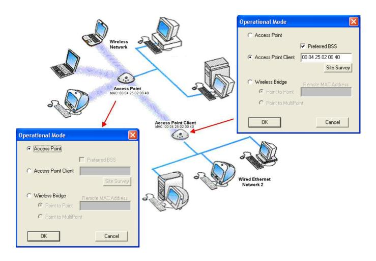
Figure 4-2 Access Point Client
