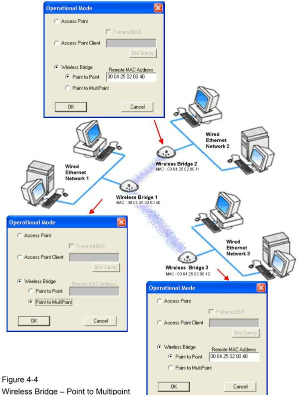
For each mode you can either view or modify the Wireless LAN parameters of the Wireless Operational Settings windows. In the **Operational Mode** Window there are the following parameters.
