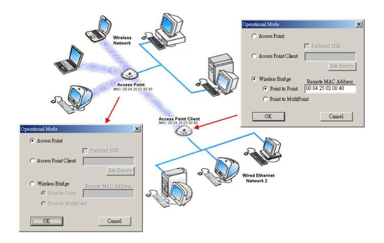
Figure 3-2 Access Point Client
