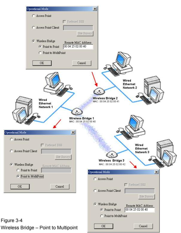
For each mode you can either view or modify the Wireless LAN parameters of the Wireless Operational Settings windows. In the **Operational Mode** Window there are the following parameters.
