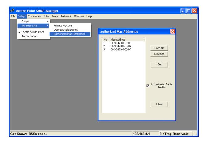
The "**Load file**" button in order to load a file with the MAC addresses that can be associated with the Access Point (Authorized MAC Addresses).
