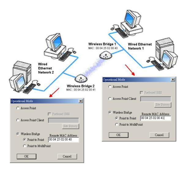
Figure 3-3 Wireless Bridge – Point to Point
