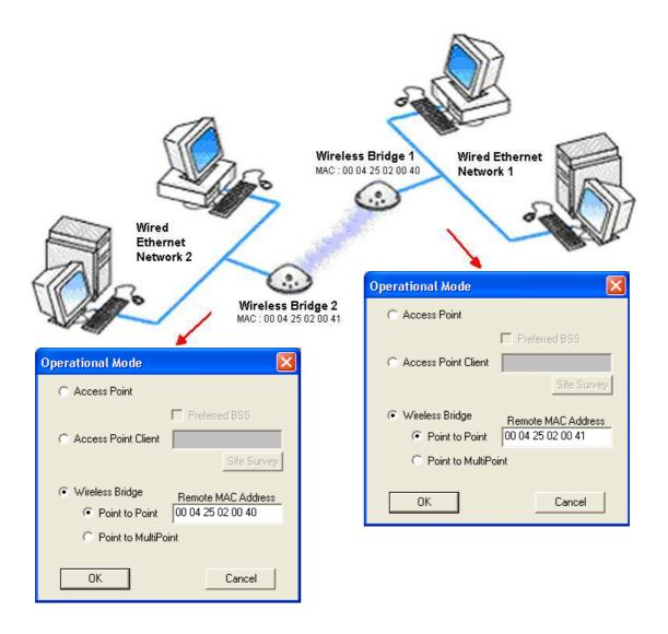
Figure 4-3 Wireless Bridge – Point to Point
